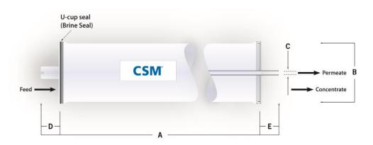
1. Each membrane element supplied with one brine seal, one interconnector (coupler) and four o-rings. 2. All RE2540 elements fit nominal 2.5 inch (64 mm) I.D. pressure vessels.
